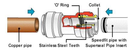
Push the pipe into the fitting, up to the pipe stop. When using correctly cut Speedfit pipe, the insertion mark on the pipe should be level with the collet head.
