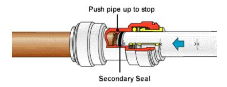
Pull on the pipe to check it is secure. It is good practice to test the system prior to leaving site or before use. Our recommended test procedure is shown in our Technical Checklist.
