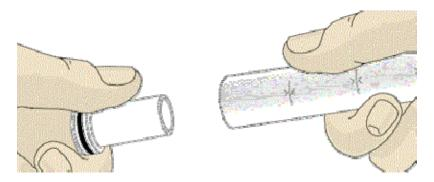
An 'O' ring on the head of the insert and the shape of the stem provide a secondary seal against the bore of the fitting. A combination of this and the main 'O' ring ensure a good connection.
