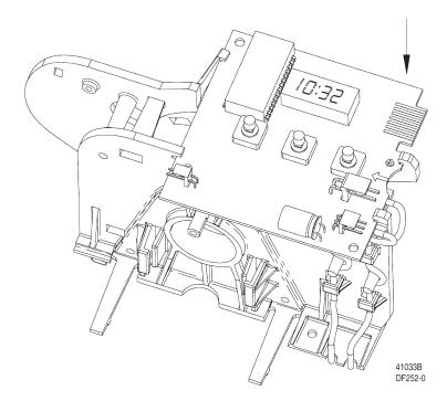
2. When all the way down, snap the circuit board into place under the notches on the right.
