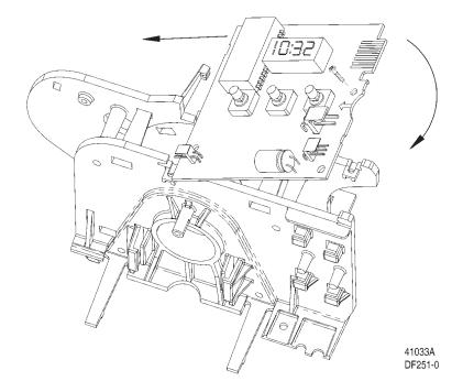
1. To insert the circuit board, align the notches on the left side of the board with the flexible finger on the power head. Apply pressure to the left while rotating the board back.
